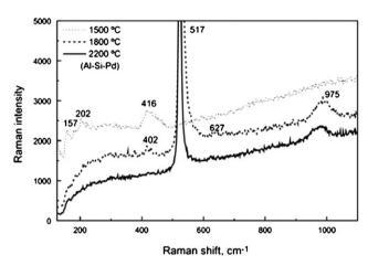
**Fig. 5** Raman spectra of pyrolytic graphite platforms containing  $100~\mu g$  each of aluminium nitrate and palladium chloride, and  $100~\mu g$  silicon, heated to 1500, 1800 and  $2200~^{\circ}C$ .
