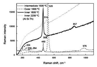
**Fig. 4** Raman spectra of three different locations of pyrolytic graphite platforms containing 100 μg each of aluminium and thorium nitrates and 100 μg silicon, heated to 1500, 1800 and 2200 °C.
