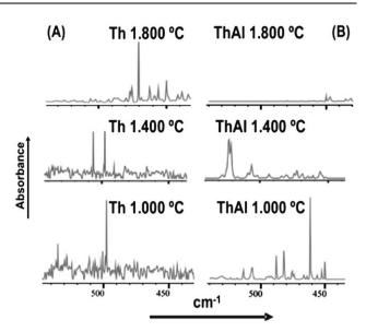
Fig. 3 FT-IR absorbance spectra of the solid residue from a large area of a graphite platform containing (A)  $100 \mu g$  of thorium nitrate and (B)  $100 \mu g$  each of aluminium and thorium nitrates heated to  $1000 \,^{\circ}$ C,  $1400 \,^{\circ}$ C and  $1800 \,^{\circ}$ C.
