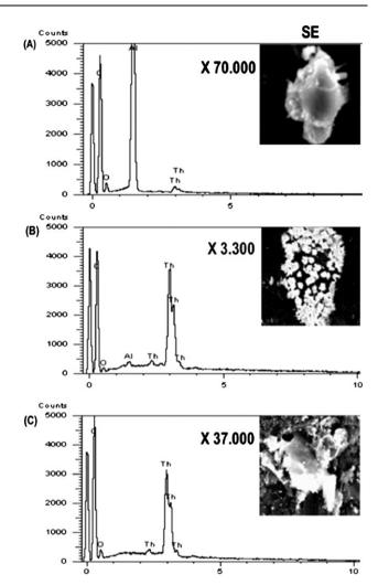
Fig. 1 ED X-ray spectra and secondary electron mappings from the (A) outer, (B) intermediate, and (C) inner regions of a non-pyrolytic graphite platform containing  $100~\mu g$  each of aluminium and thorium nitrates heated to  $2000~^{\circ} C$ .
