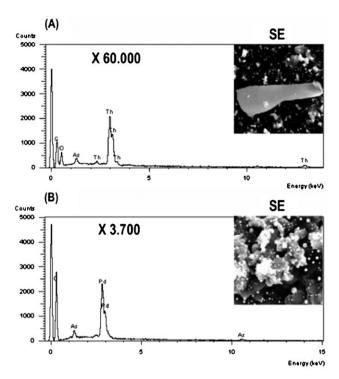
**Fig. 6** ED X-ray spectra of pyrolytic graphite platforms containing (A) 100 μg of thorium nitrate and 500 ng of arsenic and (B) 100 μg palladium chloride and 500 ng arsenic, heated to 1200 °C.
