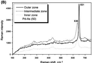
Fig. 7 Raman spectra from different locations of pyrolytic graphite platforms containing (A) 100  $\mu$ g of thorium nitrate and 500 ng arsenic and (B) 100  $\mu$ g palladium chloride and 500 ng arsenic, heated to 1200 °C.
