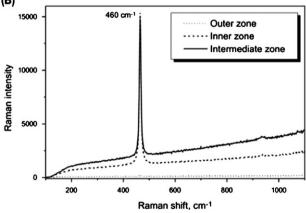
Fig. 2 Raman spectra of (A) 100  $\mu$ g of thorium (as nitrate) on pyrolytic graphite platforms heated to different temperatures and (B) 100  $\mu$ g each of aluminium and thorium nitrates on three different locations of a non-pyrolytic graphite platform heated to 1800 °C.
