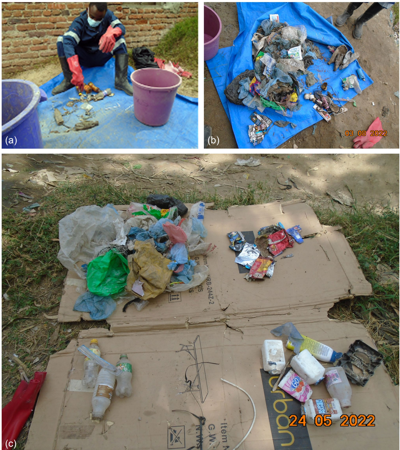
Fig. 4 Manual plastic waste quantification by polymer type (a) research team member counting plastic polymers (b) Mixed plastic polymers during manual counting (c) separated plastic polymers during counting. Source: Authors own photograph
