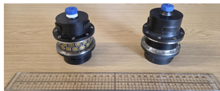
Fig. 7. Main ultrasonic bodies of the PIGs used in the practical experiments: the left device is the 32-element reference, and the right device is the 128-element phased-array. The brushes of the PIGs are not shown, as they would obscure the main ultrasonic body, the primary object of this paper.
