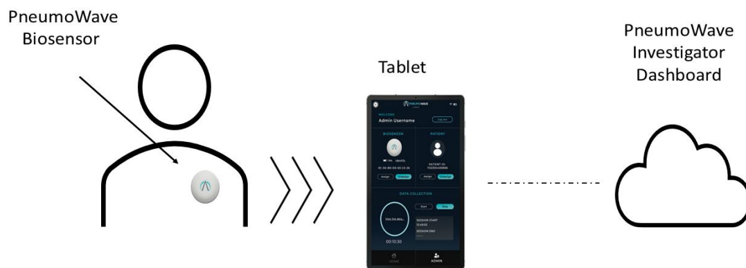
Figure 1. Hardware and software configuration for recording chest motion using the PneumoWave biosensor integrated platform of patient data capture.
