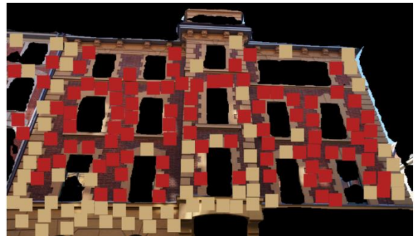
Fig. 6: Visualization of finalized clusters on a patch map after applying majority voting within each cluster to determine dominant labels; here: decorative facade with stucco (beige) and brick (red) parts
