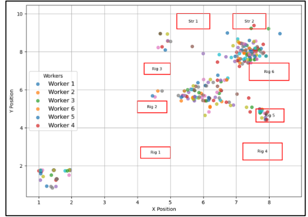
Figure 7. Temporal colocation of three or more workers within 0.5 m of Euclidean distance.
