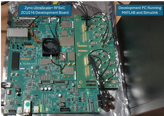
Fig. 5. Experimental Setup showing Zynq UltraScale+ RFSoc ZCU216 and Host PC.
