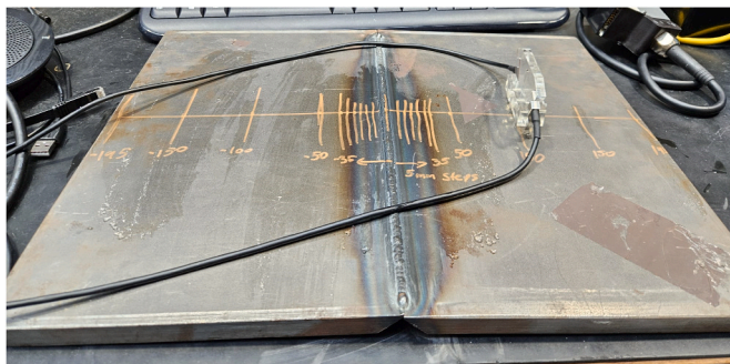
Fig. 13. Ultrasonic testing of sample.
