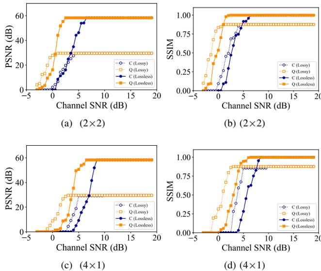
Fig. 7. Comparison of average PSNR (left) and average SSIM (right) for classical (C) and quantum (Q) systems under: (a), (b)  $2 \times 2$ , (c), (d)  $4 \times 1$  schemes with lossy (QP = 25) and lossless (QP = 100) JPEG source encoded images.
