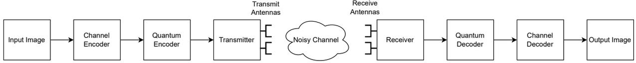
Fig. 1. End-to-end quantum communication system using MIMO technology.
