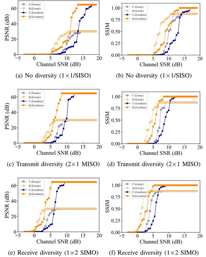
Fig. 5. Comparison of average PSNR (left) and average SSIM (right) for classical (C) and quantum (Q) systems under: (a), (b)  $1 \times 1$  SISO, (c), (d)  $2 \times 1$  MISO and (e), (f)  $1 \times 2$  SIMO diversity schemes with lossy (QP = 25) and lossless (QP = 100) HEIF source encoded images.
