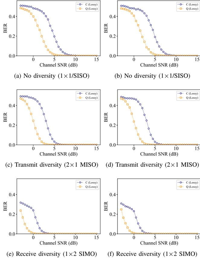
Fig. 6. BER variation for JPEG format (left) and HEIF format (right) for classical (C) and quantum (Q) systems under: (a), (b)  $1 \times 1$  SISO, (c), (d)  $2 \times 1$  MISO and (e), (f)  $1 \times 2$  SIMO diversity schemes with lossy (QP = 25) images.
