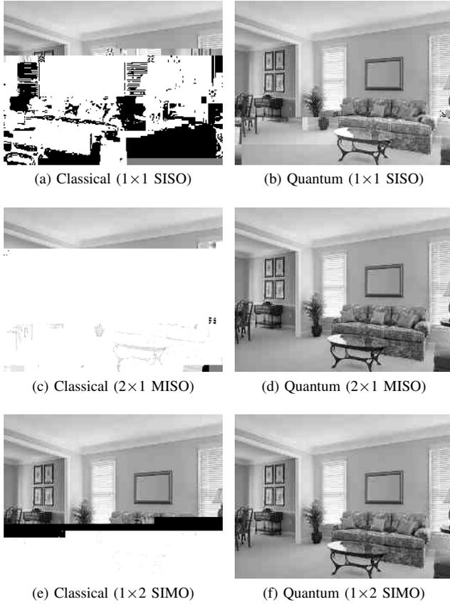
Fig. 4. Examples of received (lossy) JPEG encoded images for classical and quantum systems under each scheme. (a), (b):  $1 \times 1$  SISO with channel SNR of 10 dB; (c), (d):  $2 \times 1$  MISO with channel SNR of 7 dB; (e), (f):  $1 \times 2$  SIMO with channel SNR of 7 dB.
