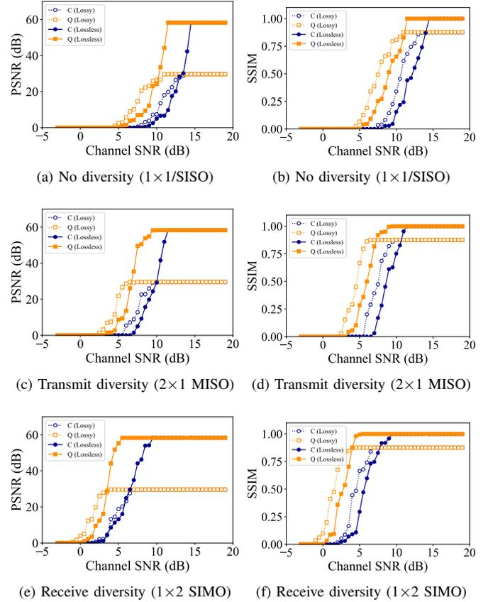
Fig. 3. Comparison of average PSNR (left) and average SSIM (right) for classical (C) and quantum (Q) systems under: (a), (b)  $1 \times 1$  SISO, (c), (d)  $2 \times 1$  MISO and (e), (f)  $1 \times 2$  SIMO diversity schemes with lossy (QP = 25) and lossless (QP = 100) JPEG source encoded images.
