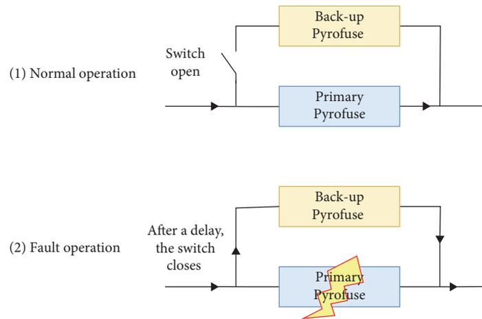
FIGURE 4: Parallel-redundant Pyrofuse set-up.
