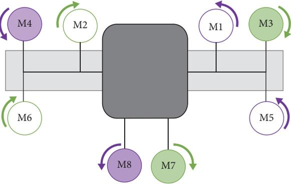
FIGURE 3: Example of lift + cruise configuration.
