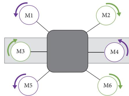
FIGURE 2: Example of vectored thrust configuration.
