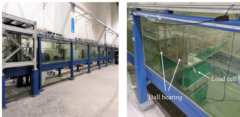
Fig. 5 Views of both the glass-walled wave flume (left panel) and the physical model in the wave flume (right panel).
