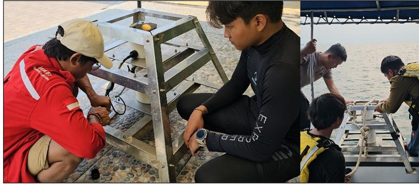
**Figure 3.** Implementation of acoustic doppler current profiler comparing wave measurement from mini wave gauge
