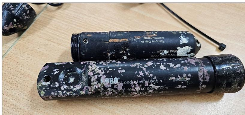
**Figure 4.** HOBO water level data logger type U20L-04
