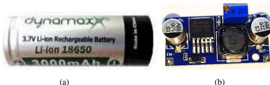
Figure 4. Li-ion battery 18650 Voltage 3,7 volt (a), Step down module LM2596 (b)
