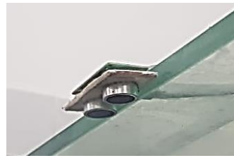
Figure 11. The ultrasonic sensor measures the wave height by counting the distance
