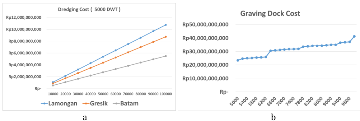
Figure 5. Empirical Graph of Investment Cost of Soil Dredging Components with Vessel Size 5000 DWT & Cost of Graving Dock Components
