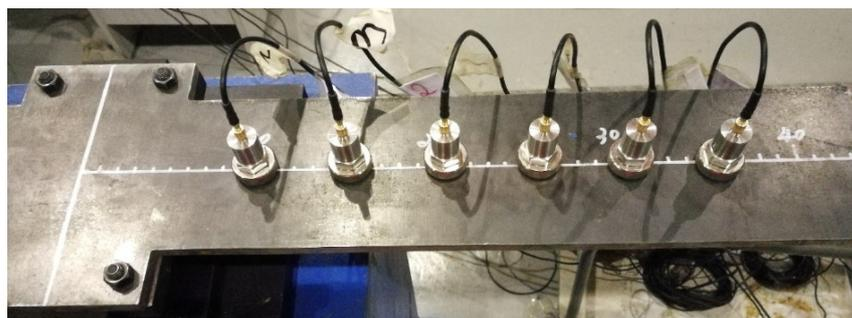
Figure 14. Layout diagram of acceleration sensors.
