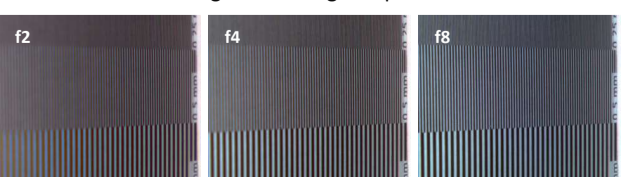
Fig. 6a. Small apertures increase depth of field and reduce chromatic effects
