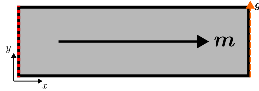
Fig. 2. Experiments of Section 5.2: View from above of the FeCoSiB bar of dimensions (20\ell_{\text{ex}}, 6\ell_{\text{ex}}, 6\ell_{\text{ex}}) .
