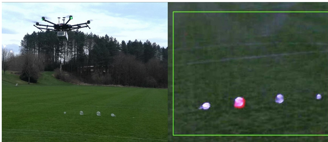
Fig. 4. The drone-mounted methane imaging system. Left image depicts the system in flight, while imaging 4 target balloons. Right image is an example frame observed from the gas imaging system from a vertical height of 3m during a fly in shot from a horizontal distance of 22m to 10m at a background light level of 52Lux. The methane filled balloon is highlighted in red in contrast to the three containing nitrogen. The methane is coloured red here to distinguish more clearly from the grass background. Due to low light intensity a 3\times gain is applied to the visible feed to increase clarity. This is an example frame from a video attached as supplementary material S1.
