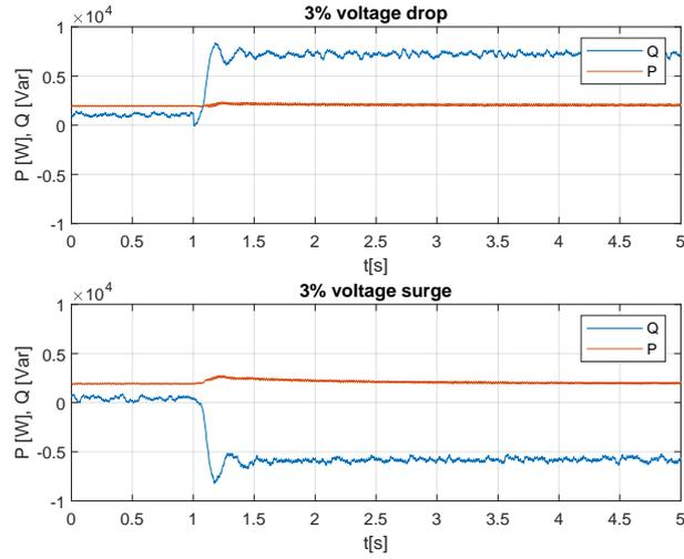
Fig. 12 Active and reactive power waveforms for the case of 2kW active power generation.
