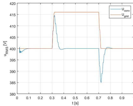
**Fig. 8** Voltage waveforms in the network and at the terminals of the converter -4% voltage surge.
