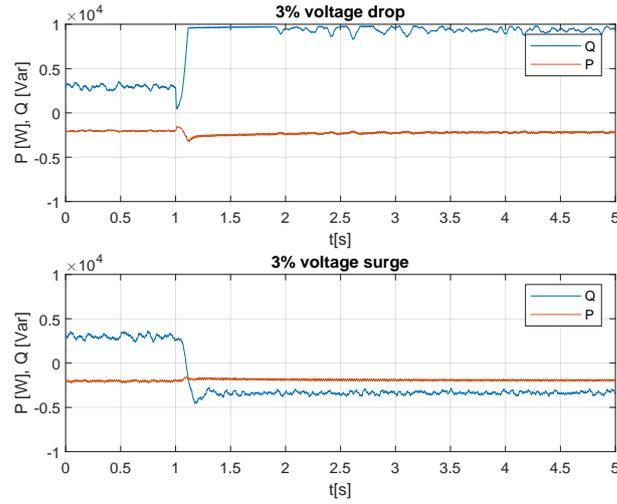
Fig. 14 Active and reactive power waveforms for the case of 2kW active power consumption.
