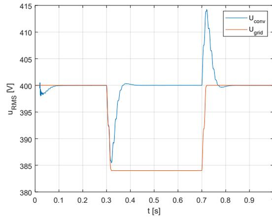
**Fig. 7** Voltage waveforms in the grid and at the converter terminals -4% voltage drop.
