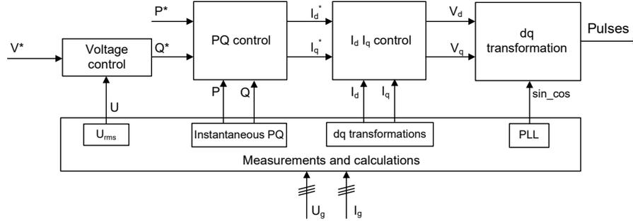
Fig. 10 Converter control system.
