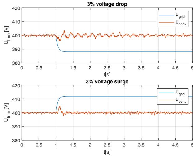
Fig. 15 Voltage waveforms for the case of zero active power.
