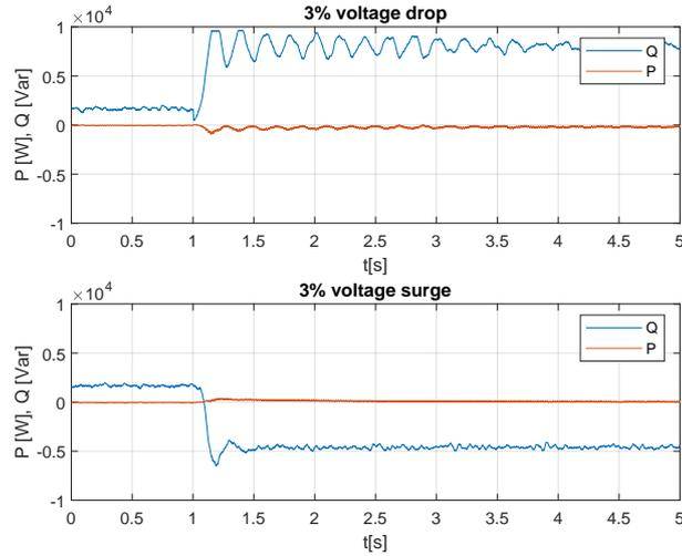
Fig. 16 Active and reactive power waveforms for the case of zero active power.
