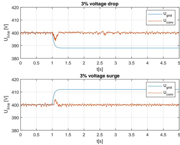
Fig. 13 Voltage waveforms for the case of 2kW active power consumption.
