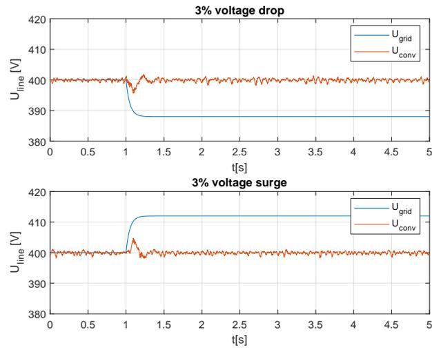
**Fig. 11** Voltage waveforms for the case of 2kW active power generation.
