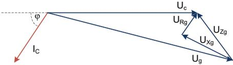
Fig. 2 Active power generation with simultaneous reactive power consumption.
