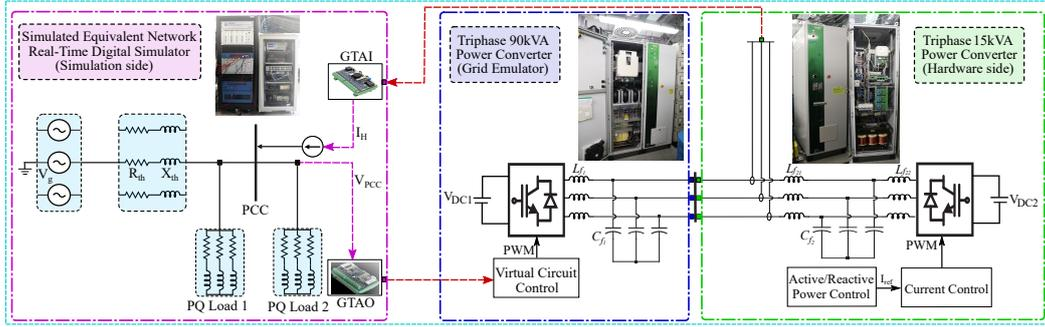
**Fig. 9** A representation of the PHIL experimental setup.
