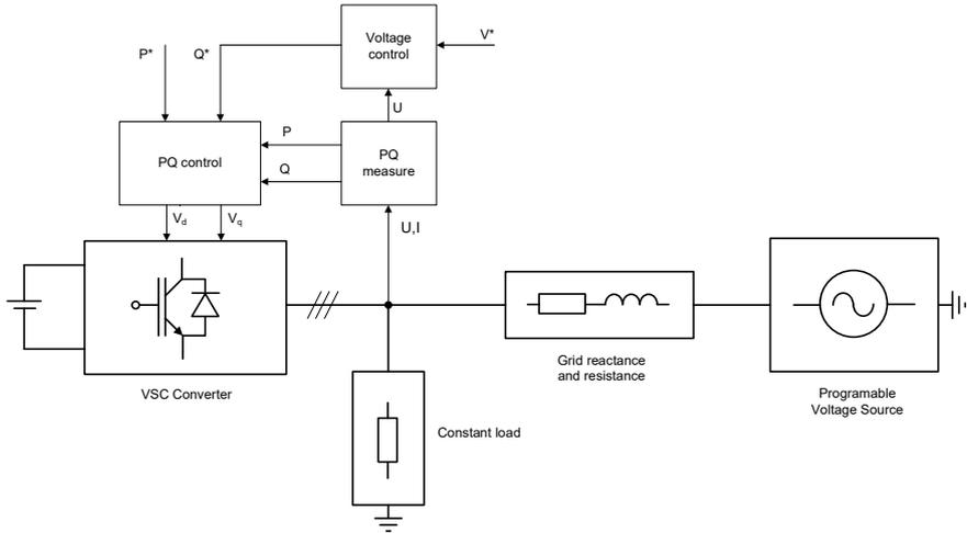
Fig. 6 Model of the system for rapid compensation of voltage fluctuations.
