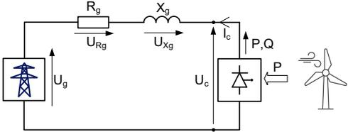
Fig. 1 Power flow and voltage drops to compensate for voltage fluctuations and reactive power.
