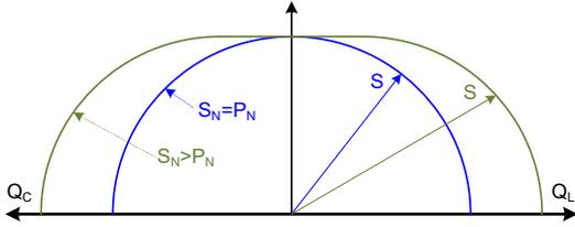
Fig. 5 Reactive power limitations due to the operating point.
