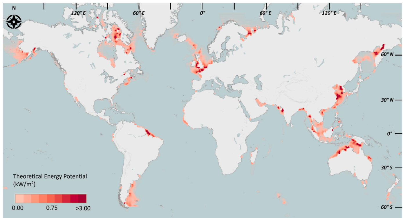
Fig. 7. | Map quantifying an upper limit for the global energy potential of tidal currents.
