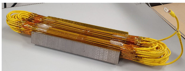
FIGURE 21. The final constructed experimental winding #9354.
