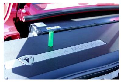
Tesla battery packs include thousands of commodity battery cells (in green). But as all laptop users know, batteries degrade over time – a potential problem for Tesla and its customers down the road. arnolddeleon/flickr, CC BY-SA
