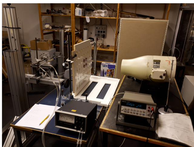
Fig. 4 | The open environment test set-up. The air flow in the direction of the eco-cooler is controlled in the experimental set-up.
