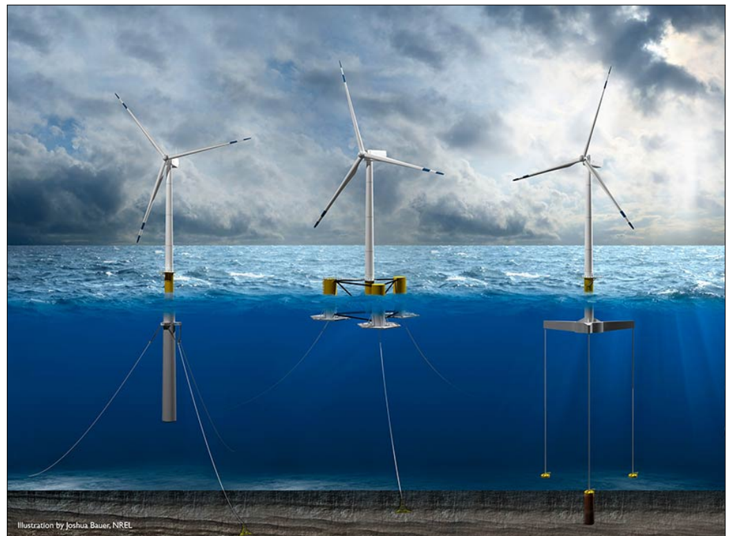
Figure 1. The three different floating platforms for offshore wind turbines. From left to right, spar-buoy, semi-submersible, and tension-leg platforms. All three foundations are tethered to the sea bed through an anchoring–mooring system. Image by Joshua Bauer, NREL [14].
