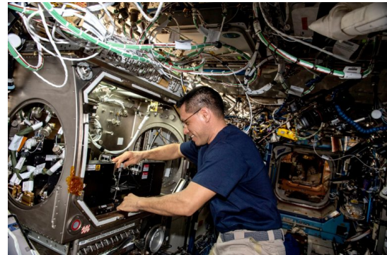
Fig. 1 - Astronaut Frank Rubio installing the PARTICLE VIBRATION Hardware into the Microgravity Science Glovebox (MSG) on board the ISS (3 rd Feb 2023).
