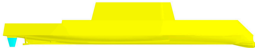
Figure 2. Geometry of the benchmark ship hull of a navy surface combatant, ONRT.
