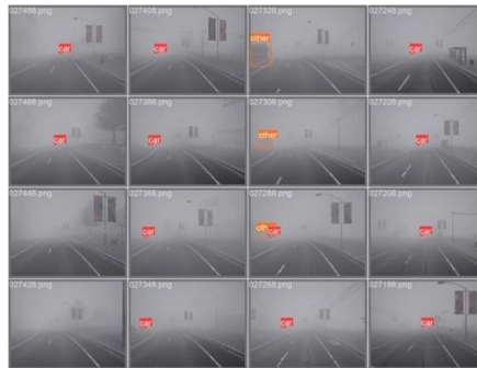
Figure 141. Detection of vehicles, the density of the fog in this photo is 100% as generated by Carla simulations
