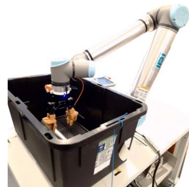
Fig. 1. Haptic Gripper mounted on UR10e Cobot for lab testing
