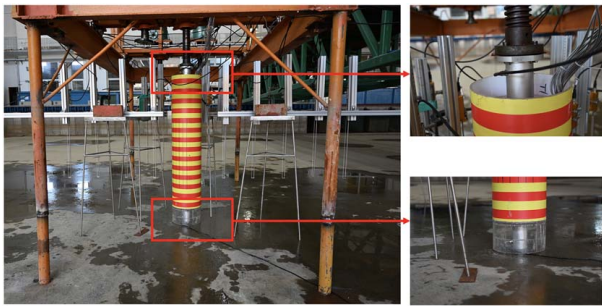
Fig. 4 The cylinder installation and force measurements
