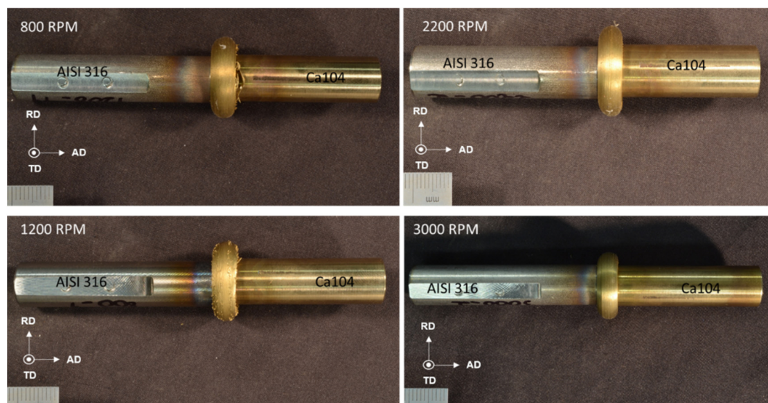
Figure 3. RFW joints of AISI316 to Ca104 utilising the capabilities of the small-scale friction welding machine. AD, TD and RD refer to the axial, radial and transverse directions, respectively.
