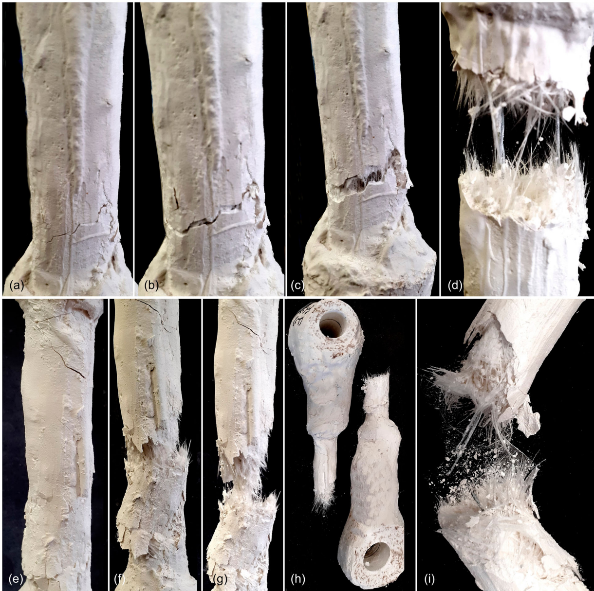
Figure 12. Failure specimens of CFG reinforced wads with steel wires – sample groups 5 and 6: looped (group 5, a – d) and looped-twisted (group 6, e – i). Group 5 looped steel wires elongated and typically supported slightly lower maximum loads but did not break (although CFG fibres did). Group 6 wires could support slightly higher maximum loads, but wires did break in addition to the CFG fibres, resulting in specimens entirely broken in two. CFG samples typically displayed less small plaster cracks in multiple locations than hessian groups, but more pronounced primary cracks prior to failure.
