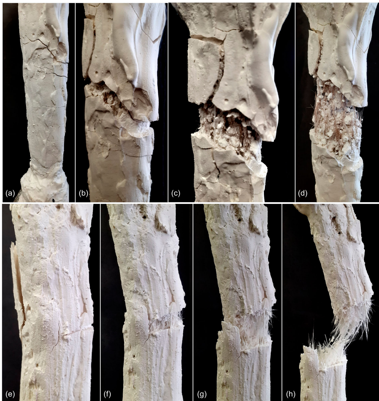
Figure 8. Failed specimens from sample groups 1 and 4, with hessian (group 1, a – d) and CFG (group 4, e – h). Hessian fibres did rupture but the wad specimen did not break entirely, continuing to function on a very small loading. CFG scrim did ultimately break the wad specimen into two.
