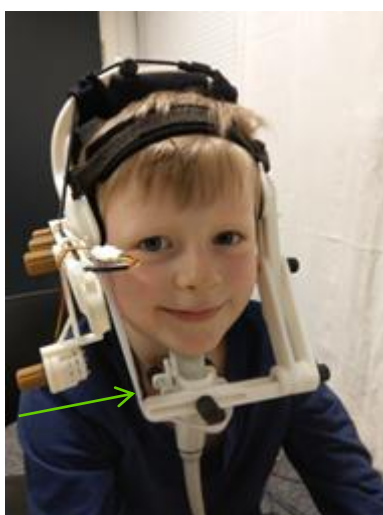
Figure 5: The Ultrafit headset worn by a 5-year-old child. Green arrow shows position of microphone.
