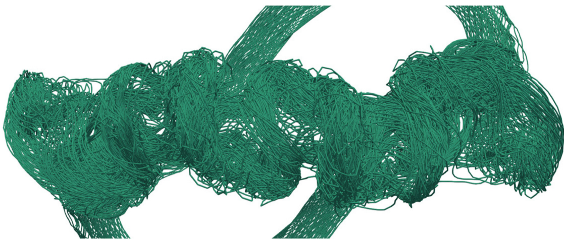
FIG. 40. Bundle link configuration with augmented circulation. An enlarged view of the emergent vortex structures generated by the Crow instability at t = 1.3689\tau_c .
