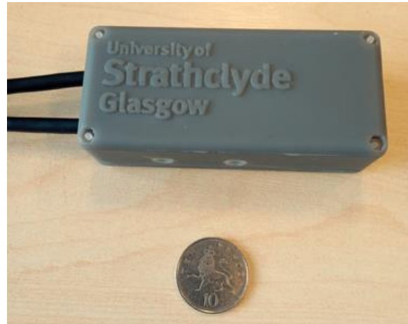
Figure 1: Portable optical magnetometer sensor head developed at the University of Strathclyde. This sensor head contains the microfabricated caesium vapour cell, VCSEL light source and analogue detector electronics. It weighs < 200 g and has a volume of 100 cubic centimetres.
