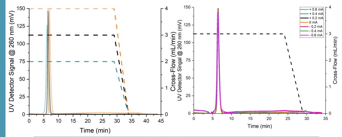
Cross-flow dependant elution times, shift by 52 seconds increasing XF from 2-4 mL/min.
