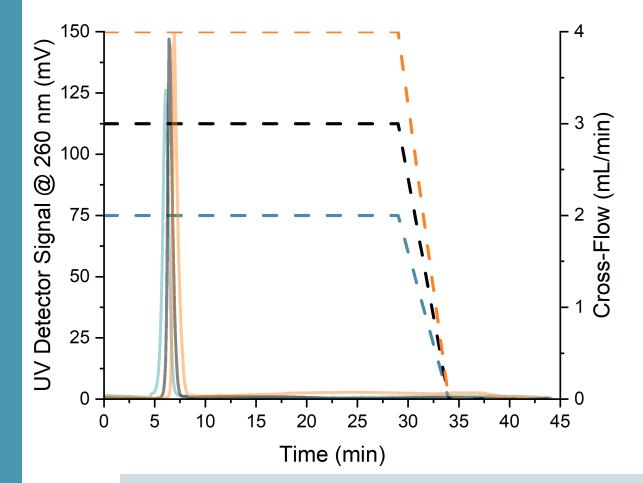
Cross-flow dependant elution times, shift by 52 seconds increasing XF from 2-4 mL/min.
