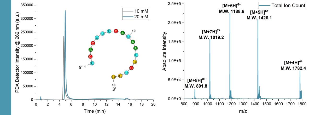
Increased retention and increased PDA detector intensity (40 %) with increased salt concentration.
