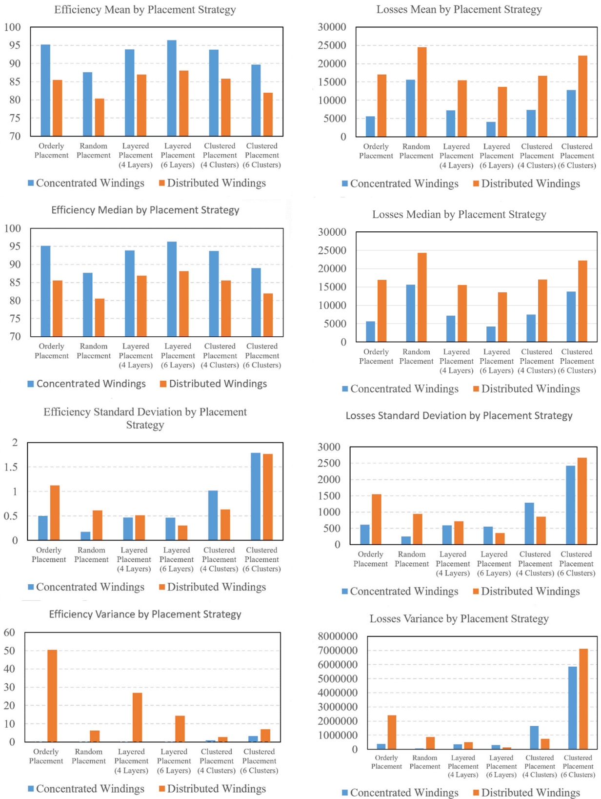
FIGURE 23. Statistical analysis graphs for the objective functions of efficiency and losses. The graphs for mean, median, standard deviation and variance by objective function are shown.
