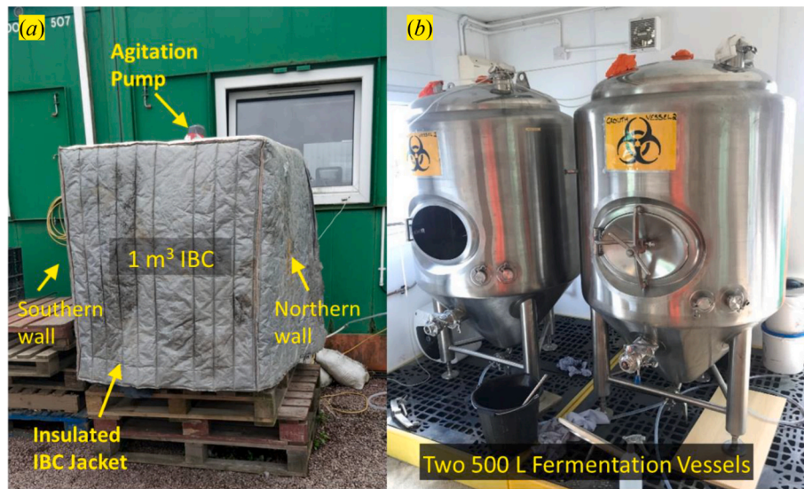
Fig. 1. Large-scale cultivation of S. pasteurii cells under non-sterile conditions in (a) 1000 L intermediate bulk container (IBC) and (b) two 500 L fermentation vessels.
