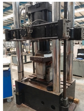
Fig. 4. (a) Schematic set up of the fatigue tests on M72 studs, (b) a picture of the fatigue test set up on a servo-hydraulic machine.
