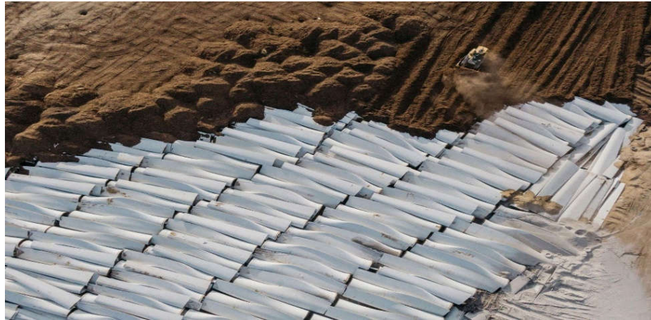
Figure 11. The impact of fabricating materials for wind turbine blades [resin/fibre glass] on decommissioning: a top view of the Casper landfill, Wyoming.
