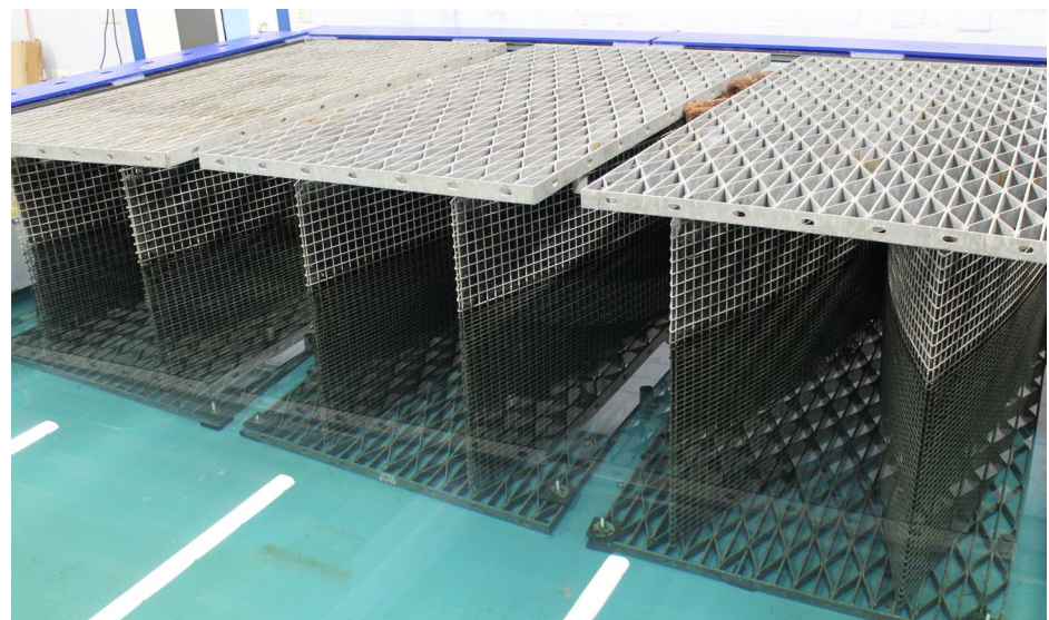
Figure 2. Wave absorbing device at the end of the wave tank.
