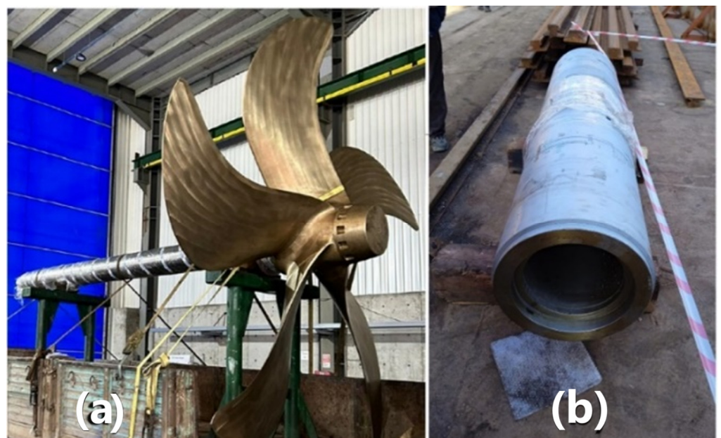
Figure 8. The new propeller and shaft manufactured and fitted (a), and the new stern tube (b).
