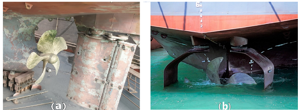
Figure 3. MV ERGE’s rudder blade(s) and propeller before (a) and after (b) the GRS retrofitting.
