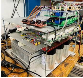
Figure 4: 20 kW 3-phase 4-wire NPC converter designed and built at UCT and the test results.
