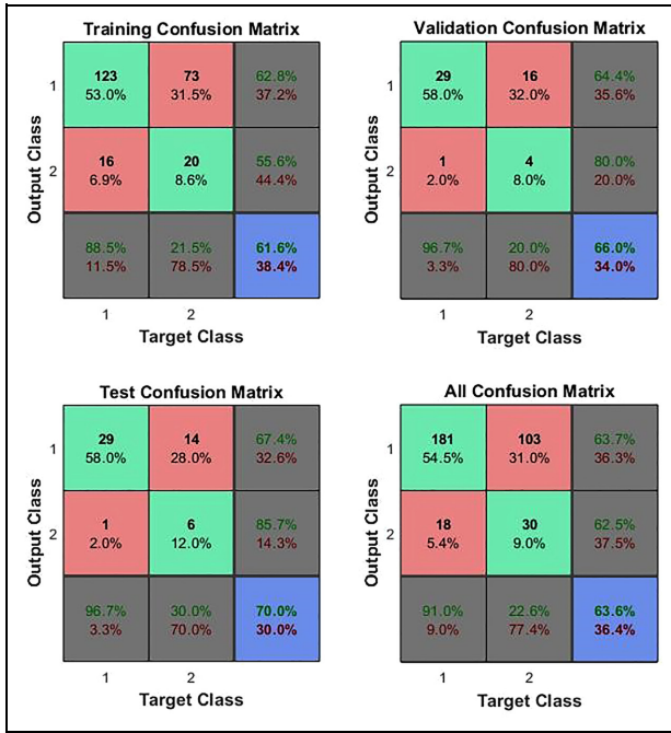
Figure 5. ANN confusion matrices for in vivo measurements on patients 11–22, assessed at either 1 or 5 Hz. Class 1 is C and Class 2 is NC and so element 1,1 represents true positives, 1,2, false positives, 2,1 false negatives and 2,2, true negatives.
