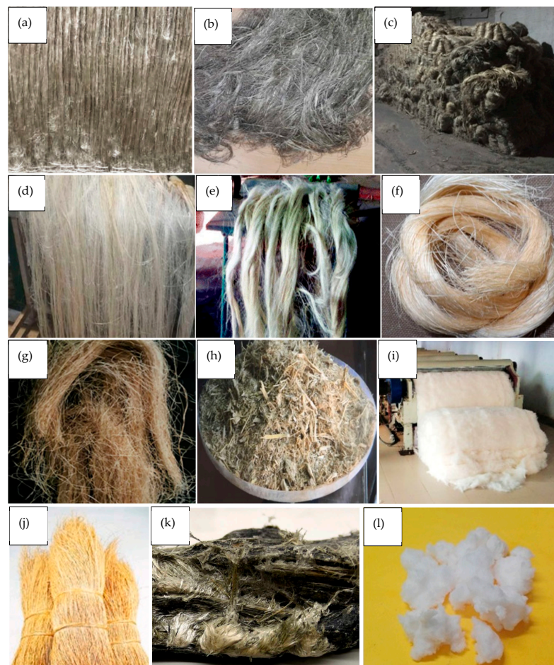
Figure 3. Extracted fibres of flax (a) [40], hemp (b) [41], jute (c) [42], kenaf (d) [42], sisal (e) [42], abaca (f) [42], bamboo (g) [43], bagasse (h) [42], cotton (i) [42], coir (j) [32], asbestos (k) [44], and regenerated cellulose fibres (l) [45].
