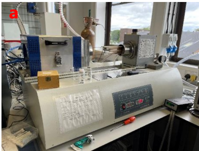
Fig. 7. Linseis system used in this study (a), measured Seebeck coefficient and electrical resistivity (b)
