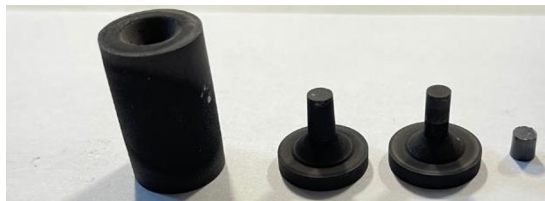
Fig. 2. Graphite die, punches and sintered part
