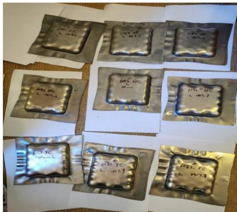
Fig. 6 Square samples from hot multi-point forming with cooling process.
