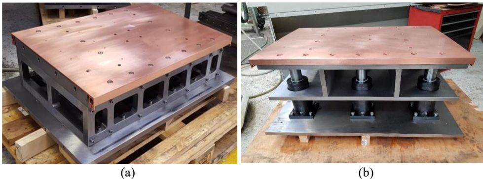
Fig. 5. Tooling used for fast contact cooling: (a) upper and (b) lower.
