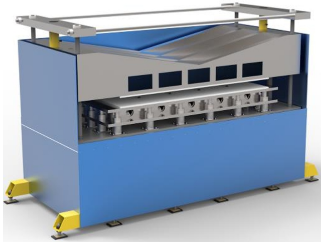
Fig. 3. Conceptual design of a contact cooling system
