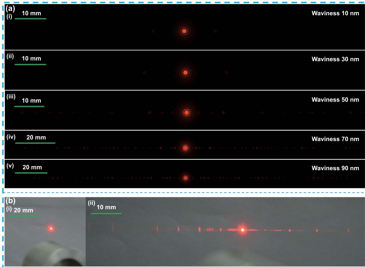
Figure 3. Influence of diamond tool cutting edge waviness on the surface diffraction effect: (a) simulation results, (b) experiment results. Reproduced from [51]. CC BY 4.0.
