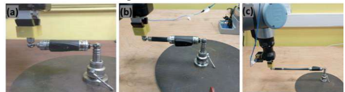
Fig. 1. Experimental setup for cobot motion in a circular path of radii (a) 100 mm (2) 150 mm (3) 300 mm
