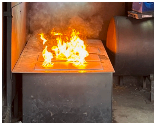
Fig. 2. Steel box used for burning samples.
