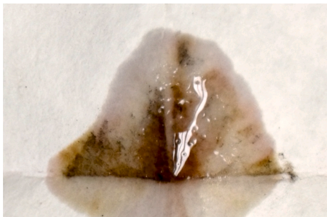
Fig. 6. “Weak” KM test result where the positive pink colour reaction was obstructed by soot.
